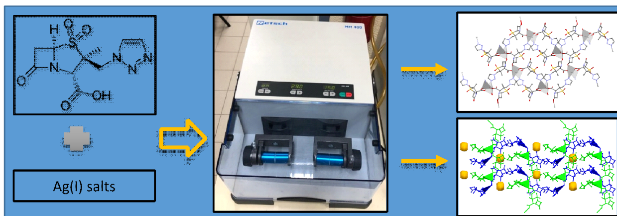
Figure 1. Scheme of the synthesis of new Ag(I)-ACFs with tazobactam by ball milling.
