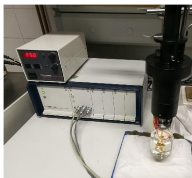
Figure 1. Thermometric 2225 solution calorimeter
